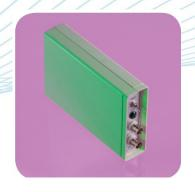
The VB/01 and VB/02 are low cost battery powered single channel IEPE signal conditioning units. Using BNC input and output they provide LED indicators for power, short circuit and open circuit checks on sensor connection. Providing a 4mA constant current supply at 18VDC they can be used with any IEPE accelerometer or other sensor.
